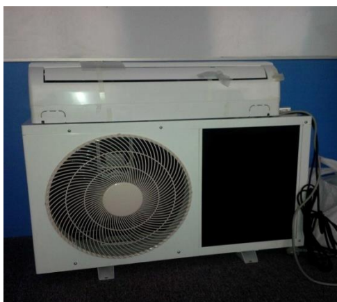
Fig. 1: Solar-assisted air-conditioning unit (left) and office building / case study (right)
