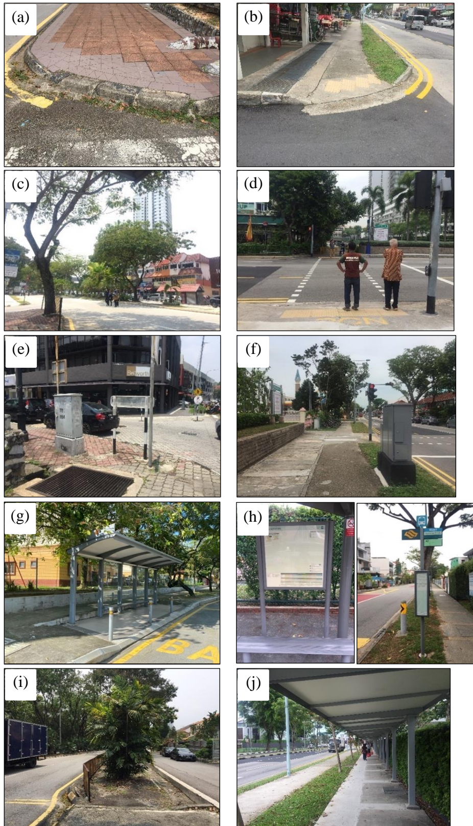
Fig. 3. Visual evidence of physical attributes between TTDI, Kuala Lumpur and Bedok, Singapore. (a) kerb step on pavement at TTDI; (b) kerb ramp on pavement at Bedok; (c) no pedestrian crossing at TTDI; (d) pedestrian crossing at Bedok; (e) obstruction on pedestrian pavement at TTDI; (f) buffer zone for amenities and street furniture at Bedok; (g) no bus stop information at TTDI; (h) bus stop information at Bedok; (i) poor pavement condition with landscape obstruction and without walkway shelter; (j) good pavement condition with walkway shelter at Bedok.
